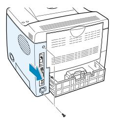
4 Remove the two screws and the bracket from the control
